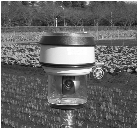
Figure 1. A standard Field Server. Field Servers can be equipped with monitoring sensors and control switches.
