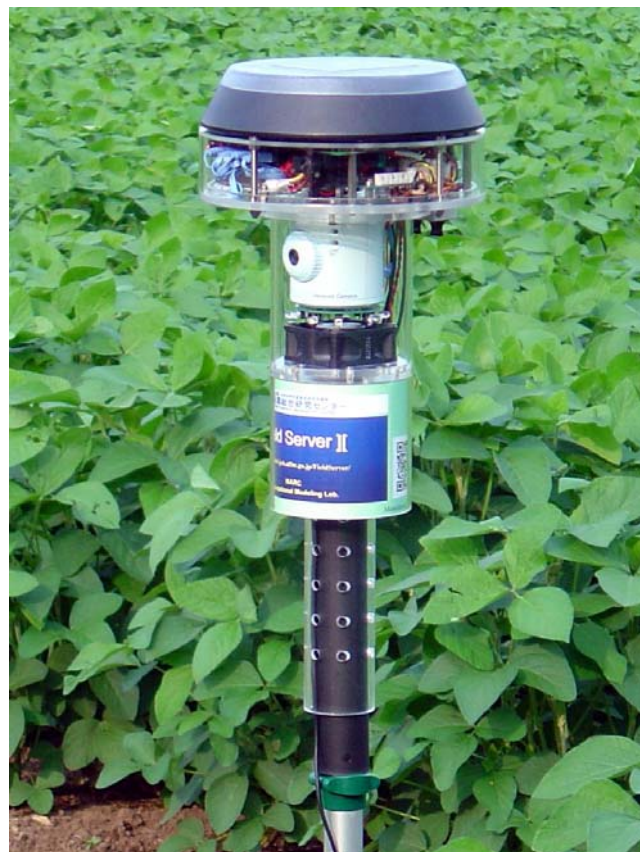
Fig. 1 Field Monitoring Server consists of a solar cell, Web server card, Wi-Fi access-point card, sensors, a network camera and fan. They are connected by wireless LAN.
