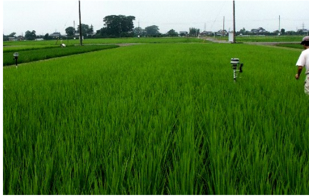
Fig. 4 Full-wireless Field Monitoring Servers installed in a paddy field.
