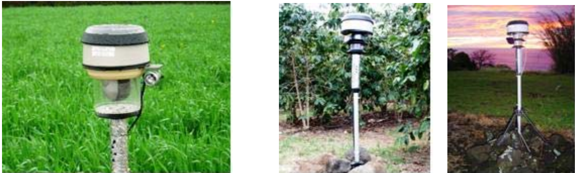
(a)FMS at upland farm in Tsukuba, Japan (b) FMS at UCC coffee Farm in Kona, Hawaii USA Figure 1. Standard type of FMS, which require DC12V power supply to maintain backbone connection and hotspot with Wi-Fi(IEEE802.11b/g).
