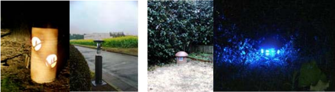
(a) Access point garden-lighting FMS (b) Client-connection garden-lighting FMS at a garden Figure2. Garden-lighting FMS. To produce backbone and hotspot in fields, sometime FS must be installed at gardens around private houses or buildings. Garden-lifting type FMS (a) can fit to such locations. Client-connection garden-lighting FMS (b) can be easily installed at a hotspot and function as a garden light controlled remotely by Fieldserver-Agent.
