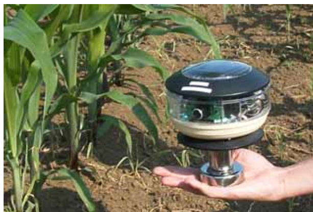
Fig.1. Field Server as a Web-based sensor node.
