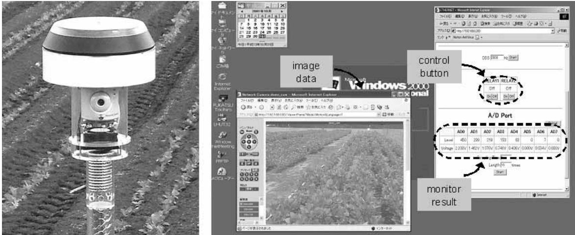
Figure 1. Field Server as a Web-based sensor node.
