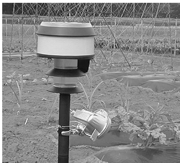
Fig. 1. A standard Field Server. Field Servers can be equipped with sensors, for example for temperature, humidity and solar radiation, and with switches for heaters, water sprinklers, etc.
